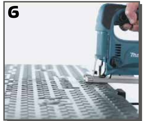
The Cross 5 can be cut into two using a compass saw. This allows you to create even more crossover structures.
